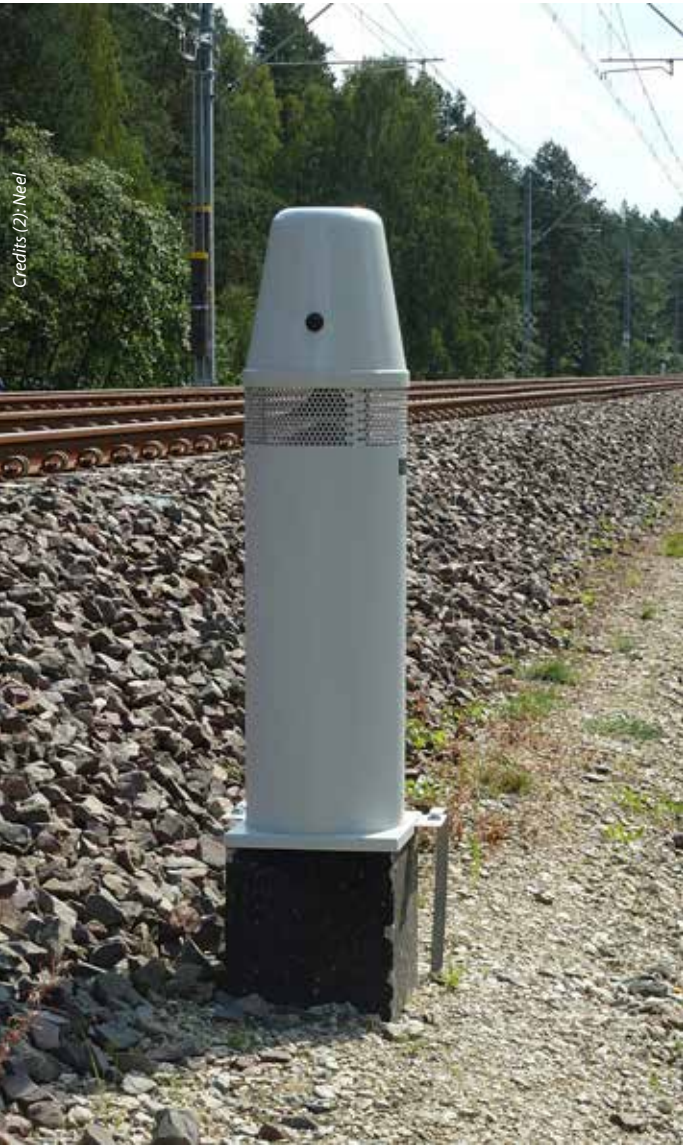
A close-up view: an acoustic warning station from the company NEEL.
